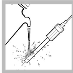
3. Rinse the probe with deionized water. Put it in the standard solution so that the temperature sensor is completely submerged.
