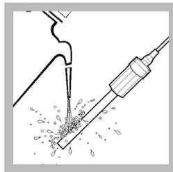
2. Rinse the probe with deionized water and blot dry with a laboratory wipe.
