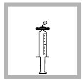
**8.** Hold the syringe with the filtration attachment pointing upwards and **slowly press the liquid upwards** until the membrane filter is wetted.
