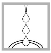
**14.** With a 1 mL plastic dropper, add 1.0 mL of pPb-4 Neutralizer Solution to the bottle.
