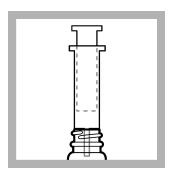
**13.** Let the Eluant Solution drip slowly from the Extractor. When the flow stops, fully compress the absorbent pad.
