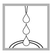
**26.** Add 3 drops of pPb-6 Decolorizer Solution to the sample cell.
