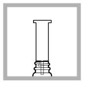
**8.** Put a new Fast Column Extractor on top of the second 125-mL sampling bottle. A new extractor is necessary for each test procedure.
