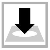
**22.** Insert the prepared sample into the cell holder. Point the diamond mark on the sample cell toward the keypad.
