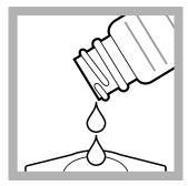
10. Slowly pour the prepared sample into the center of the Column Extractor. Wait for the sample to flow through. It is expected that the sample solution flows slowly (2 drops per second) through the column. Keep the level of the sample solution just above the cotton plug.
