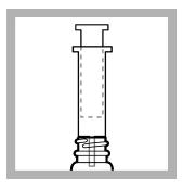
11. After the flow stops completely, fully compress the absorbent pad in the Extractor with the plunger. Safely discard the contents of the bottle. Make sure that the absorbent pad stays at the bottom of the Extractor when the plunger is removed. If the cotton plug moves up the column, push it back to the bottom with a clean, blunt rod.
