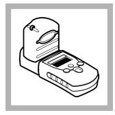
**23.** Install the instrument cap over the cell holder.
