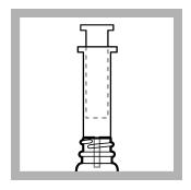
9. Soak the cotton plug with deionized water, then compress it with the plunger. Make sure that the cotton plug fits snugly against the inner wall of the column. Remove the plunger.
