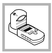
**30.** Install the instrument cap over the cell holder.
