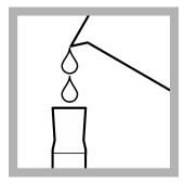
**1.** Fill a plastic graduated cylinder with 100 mL of the sample.
