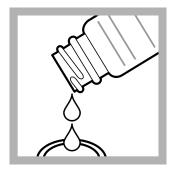
**18.** Fill a sample cell to the 10-mL mark with the solution.
