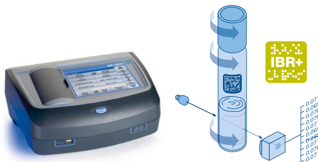
Left: the DR3900 spectrophotometer Right: the 10-fold measurement, which turns the cuvette while taking intermittent measurements
