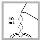
2. Fill two sample cells with 10 mL of sample. Label one cell as the sample. Label the other cell as the blank.
