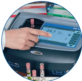
Fig. 2: Spectrophotometer for the precise evaluation of LANGE cuvette tests, e.g. for nitrogen analysis
